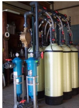
FSV-18 Six-Vessel System 18" Vessels, 20 GPM each
