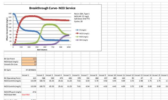
Figure 1- Example of vessel staggering in nitrate service
