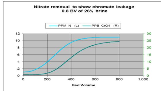
Figure 8- Breakthrough curve of NO3 and CrO4 on nitrate selective resin.
