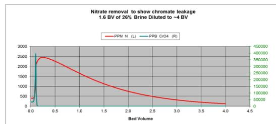
Figure 9- Regeneration curve showing sharp CrO4 removal peak.
