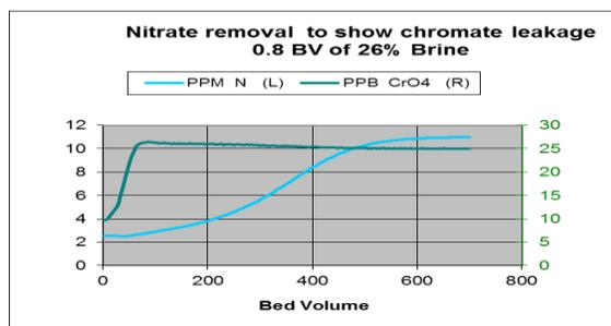
Figure 10- Breakthrough curve of NO<sub>3</sub> and CrO<sub>4</sub> on perchlorate selective resin.
