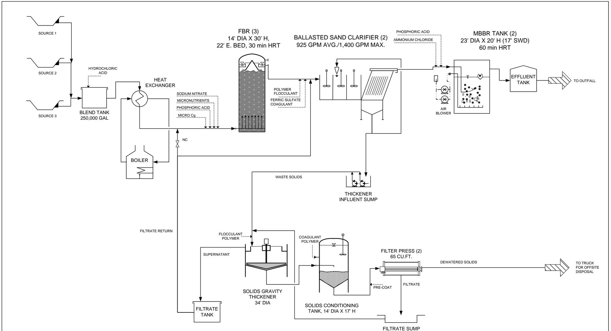
Figure 1. Process Flow Diagram – Selenium WTP
