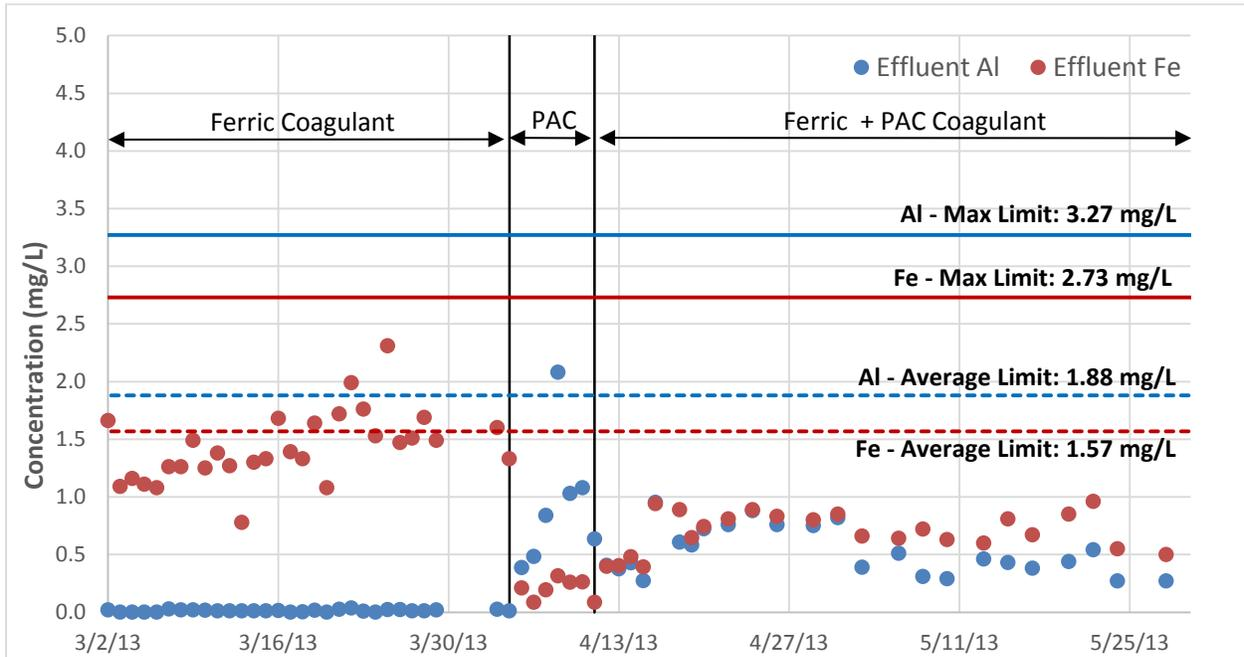
**Figure 10. WTP Initial Operations – Effluent Iron, Aluminum Data**
