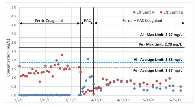
Figure 10. WTP Initial Operations – Effluent Iron, Aluminum Data
