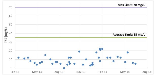
with some additional solids polishing in the MBBR tanks through settling thereby meeting compliance for not only TSS but also total selenium at the final discharge location.
