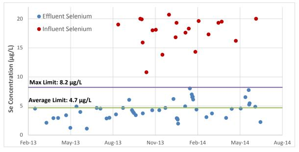
Figure 12. WTP Selenium Removal Performance
