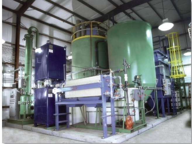
FBR system treating aniline- and nitrobenzene-contaminated wastewater in New Jersey. This technology has been certified by the State of New Jersey's DEP Innovative Environmental Technology Certification Program.
