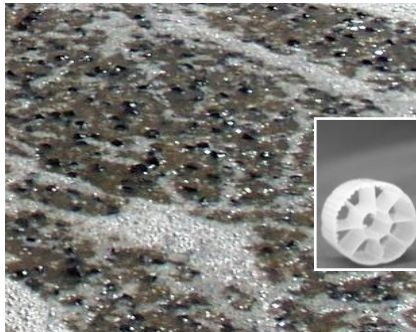
Close-up of reactor showing suspended media
