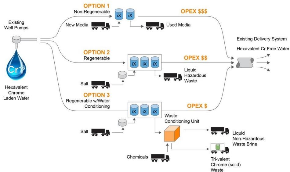
Envirogen ion exchange systems can be configured to remove a target contaminant or a combination of contaminants. This is an important feature for applications with multiple anionic contaminants, eliminating the need to employ multiple treatment technologies.
