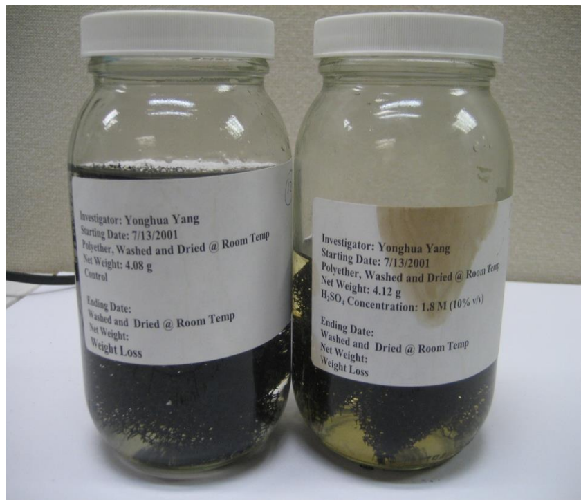
Control and Acid bottles after 11 years, 10 months
