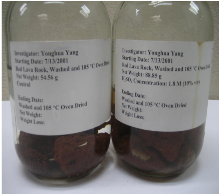
Control and Acid bottles after 11 years, 10 months
